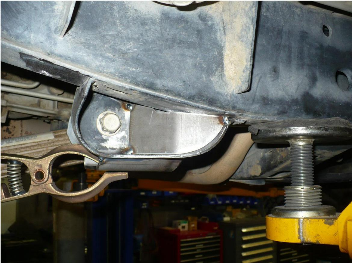
6) Next weld the seam, shown below in red, on the front most part of the stock lower control arm mount.
